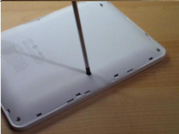
Using jewellers screwdrivers, undo the retaining screws from the back cover and place them in a safe place
