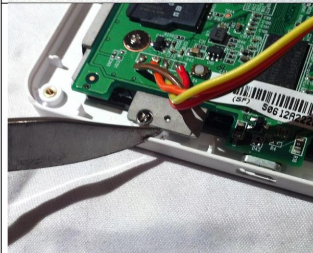
Cut the Kobo housing neatly so that the cable run out of the housing from the corner to where the GPS will be mounted
