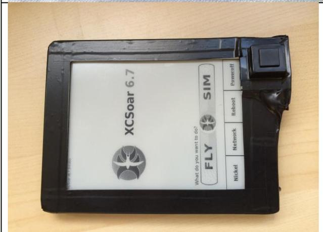
Afix the GPS unit to the outside of the Kobo using the plastic housing it came in. I have used insulating tape to hold the GPS cover in place, and to provide extra bonding between the Kobo back cover and the main Kobo unit.
